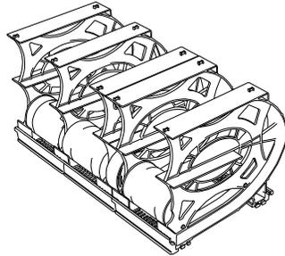
2. Finally, using the numbers on the top and bottom side of the bracket, attach the remaining 2 bracket sets to the top of the CanSolidator in the corresponding bracket holes. Attach the front bracket right side up (same as lower brackets) and the rear bracket upside down. When this is complete, the CanSolidator is ready to be filled with cans.
